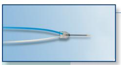
Membrane material, Cut-off Membrane Length Membrane Diameter Stainless steel shaft diameter Shaft length Inlet internal volume Outlet internal volume 200 mm Inlet tubing (blue) 200 mm Outlet tubing (transp.) Cuprophane, 6kDa 1 and 2 mm 0.24 mm 0.38 mm 7 mm negligible 3 µL
