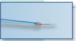
Membrane material, Cut-off Membrane Length Membrane Diameter Stainless steel shaft diameter Shaft length Inlet internal volume Outlet internal volume 200 mm Inlet tubing (blue) 200 mm Outlet tubing (transp.) PAES, 20 kDa; PES, 100kDa 1 and 2 mm 0.5 mm 0.4 mm 7 mm negligible 3 µL 3.6 µL
