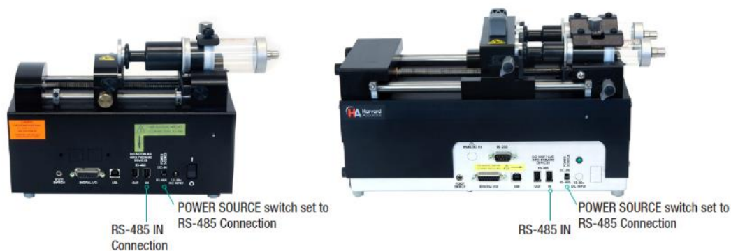
Pump 11 Elite/Pico Plus Elite (left) & PHD ULTRA™ (right) syringe pumps showing RS-485 IN connection and POWER SOURCE switch.
